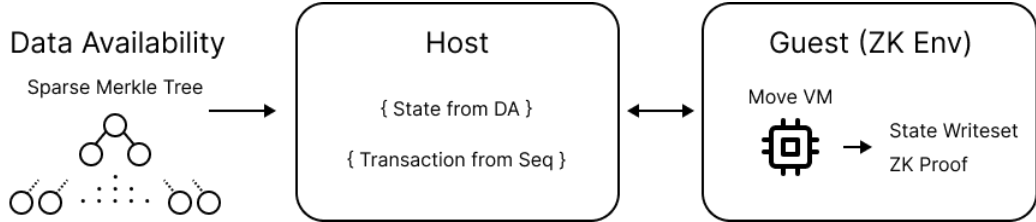
(a) Step 1: Guest executions receive state and transaction data to run Move VM, producing state writeset and ZK-Proof outputs.
